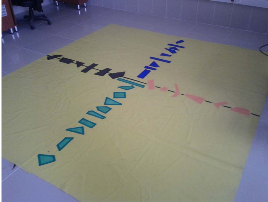
Fig. 75. Colored and randomly shaped labels on the operating floor
