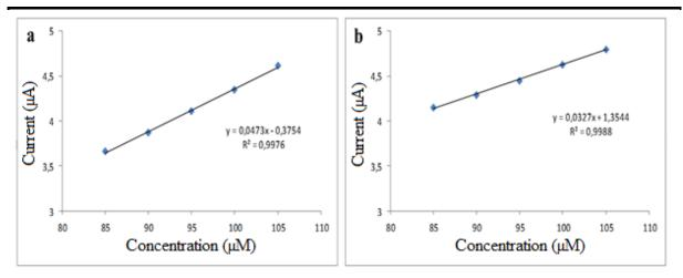
Figure 9. Calibration Curves of 5% GO/PI Composite Electrode a) for MET and b) for DP Response.
