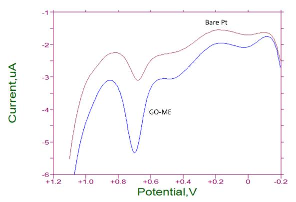
Figure 5. DPV Curves of 60  $\mu$ M of MET in PBS Buffer (pH 7.0) at the bare Pt Electrode and at the Electrode (GO-ME) Modified with 10  $\mu$ L of 5% GO/PI Composite.
