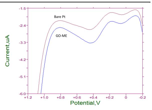
Figure 3. DPV Curves of 60  $\mu$ M UA in PBS Buffer (pH 7.0) at the Bare Pt Electrode and at the Electrode (GO-ME) Modified with 10  $\mu$ L of 5% GO/PI Composite.
