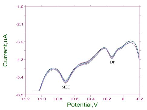
Figure 10. The Repeatability Responses of 5% GO/PI Electrode for 130  $\mu$ M MET and 80  $\mu$ M DP in the Presence of 80  $\mu$ M UA.
