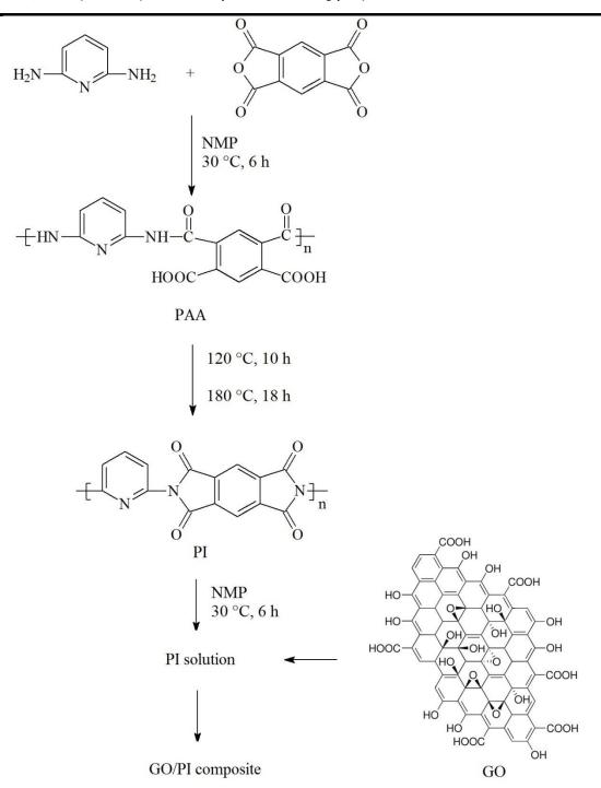
Figure 1. Preparation of the GO/PI Composite Structure.
