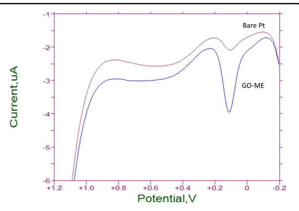
Figure 4. DPV Curves of 60  $\mu$ M DP in PBS Buffer (pH 7.0) at the Bare Pt Electrode and at the Electrode (GO-ME) Modified with 10  $\mu$ L of 5% GO/PI Composite.
