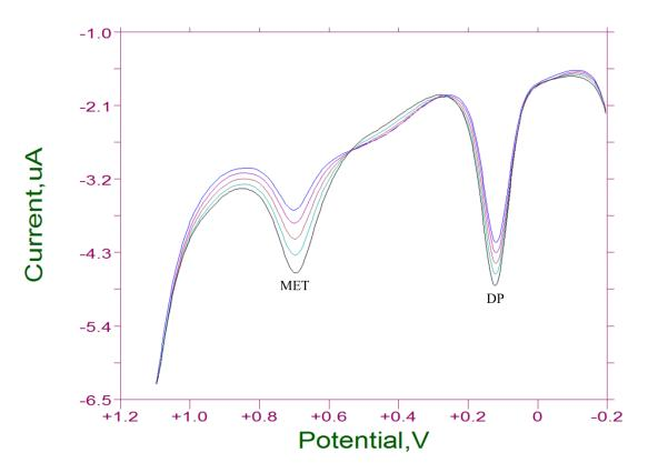
Figure 8. DPV Curves of the 5% GO/PI Composite Electrode in Various Concentrations of DP (80; 85; 90; 95; 100; 105  $\mu$ M) and MET (80; 85; 90; 95; 100; 105  $\mu$ M).
