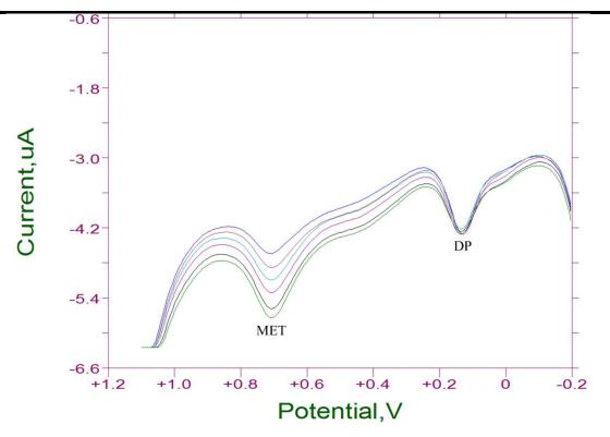
Figure 6. DPV Curves of 5% GO/PI Composite Electrode for Various Concentrations of MET in the Presence of 80 µM UA and 80 µM DP. (Melatonin: 80; 90; 100; 110; 120; 130 µM ).
