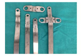
Figure 1. Visual of macroscopic surface defects of explanted pectus bars
