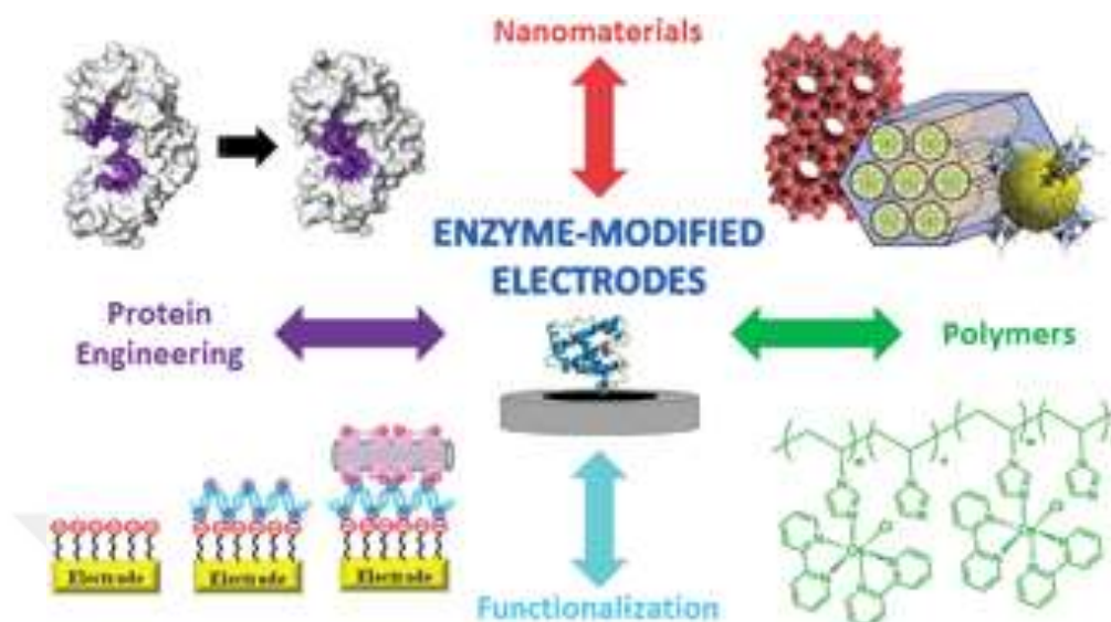
Figure 4 : Integration scheme of enzyme modified electrochemical biosensor (Pinyou et al. 2019)
