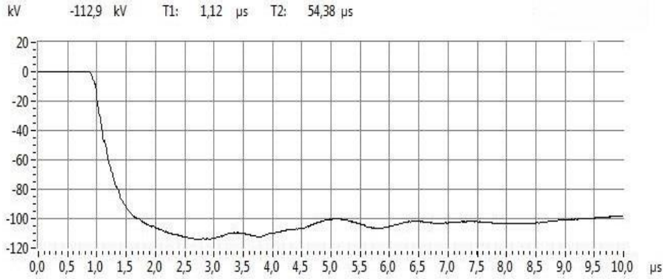
Fig. 17: Waveshape 72128072 Timsan 1000 kVA Terminal C tap 6 RFW 65%
