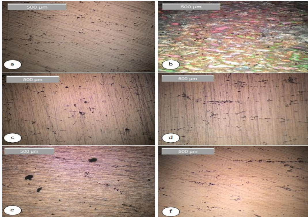
Figure 7. Microstructure images of the solution process with a waiting time of 2 hours at different temperatures a) 400 °C , b) 420 °C, c) 440 °C, d) 460 °C, e) 480 °C, f) 500 °C
