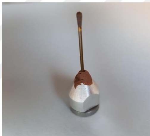
Figure 24. A sample in the Kapton tube placed on the sample holder for the powder diffraction test.
