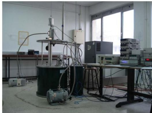
Őekil 4. 6 : Vibrating Sample Mahnetometer (VSM) sistemi (Kolat, 2007)
